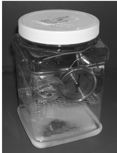
Figure 1. Sealed container with J. virginiana leaves suspended above saturated salt solution.
